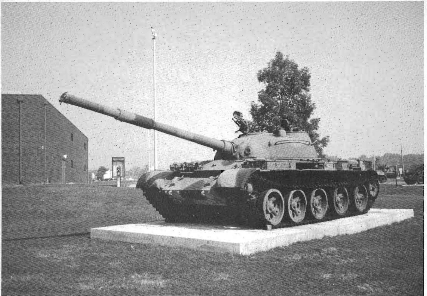
A view of the T-62M currently preserved at the Ordnance Museum. The distinctive 12.7mm DShK machine gun mount on the loader's hatch on the right side of the turret is obvious in this view. Along with an M1 Abrams and a Bradley IFV, the T-62M guards the Museum front and welcomes its visitors (Steven Zaloga)
